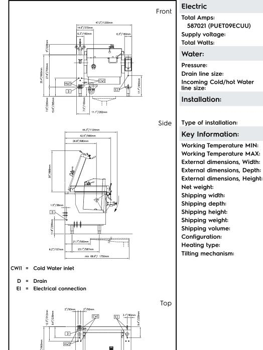
43 A 208 V/3 ph/60 Hz 15.5 kW 29-87 psi (2-6 bar) 1/2" 1/2" FS on concrete base;FS on feet;On base;Standing against wall 122 °F (50 °C) 482 °F (250 °C) 47 1/4" (1200 mm) 35 7/16" (900 mm) External dimensions, Height: 27 9/16" (700 mm) 529 lbs (240 kg) 51 9/16" (1310 mm) 49 5/8" (1260 mm) 58 1/4" (1480 mm) 1003 lbs (455 kg) 86.26 ft<sup>3</sup> (2.44 m<sup>3</sup>) Rectangular; Tilting Direct Automatic
